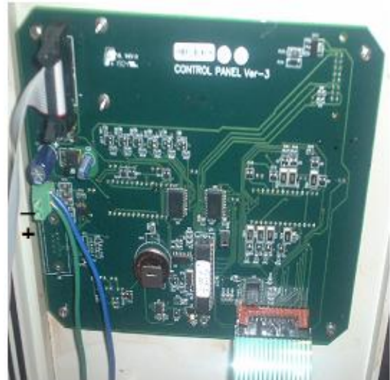
Figure 2: Connection of RS485 wire to Controller Control Panel
